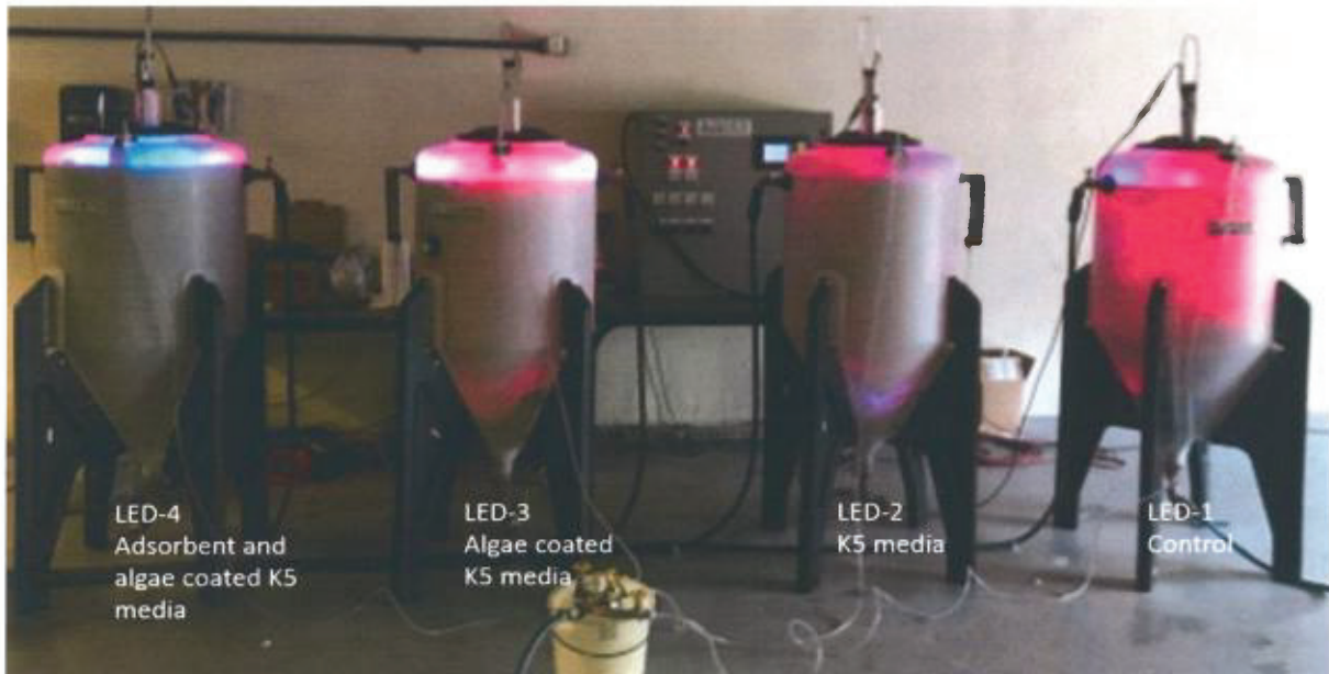
FIGURE 1: BENCH-SCALE ALGAL BIOREACTOR SETUP AT THE URBANA-CHAMPAIGN SANITARY DISTRICT WASTEWATER PLANT
