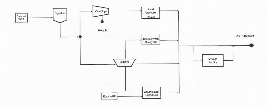
FIGURE 3: STICKNEY WATER RECLAMATION PLANT OPERATIONAL FLOW CHART FOR SECOND QUARTER 2017
