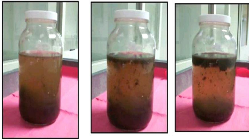
FIGURE 13: PHOTOS OF THE MIXED LIQUOR DURING PERIODIC SETTLING TESTS AT SETTLING TIMES OF FIVE, EIGHT, AND FIFTEEN MINUTES, RESPECTIVELY
