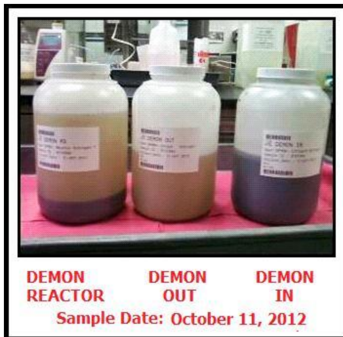
FIGURE 12: PHOTO OF THE OCTOBER 11, 2012, SAMPLES INDICATING HIGH SOLIDS ENTERING THE DEMON ® PILOT
