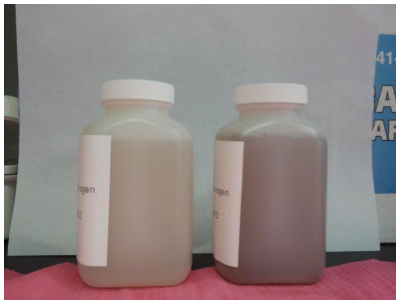
FIGURE 14: NORMAL EFFLUENT SAMPLE (LEFT) AND SOLIDS WASH-OUT EFFLUENT SAMPLE (RIGHT) FROM THE DEMON ® PILOT
