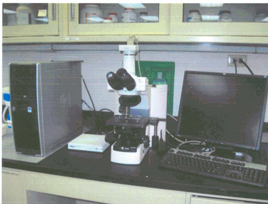
B. Nikon Eclipse 80i Digital Imaging System Which Includes a Research Microscope That is Optimized for Digital Imaging.
