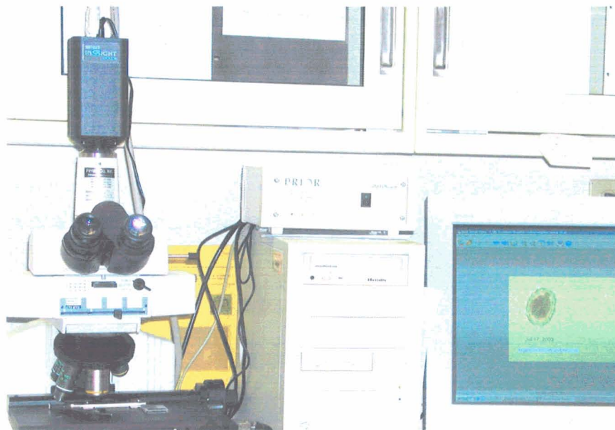
A. Nikon E600 Research Phase Contrast Microscope with a Digital Snap Video Camera Transmitting Microscopic Images from Slide to a Computer Workstation with a Metamorph Software Program.
