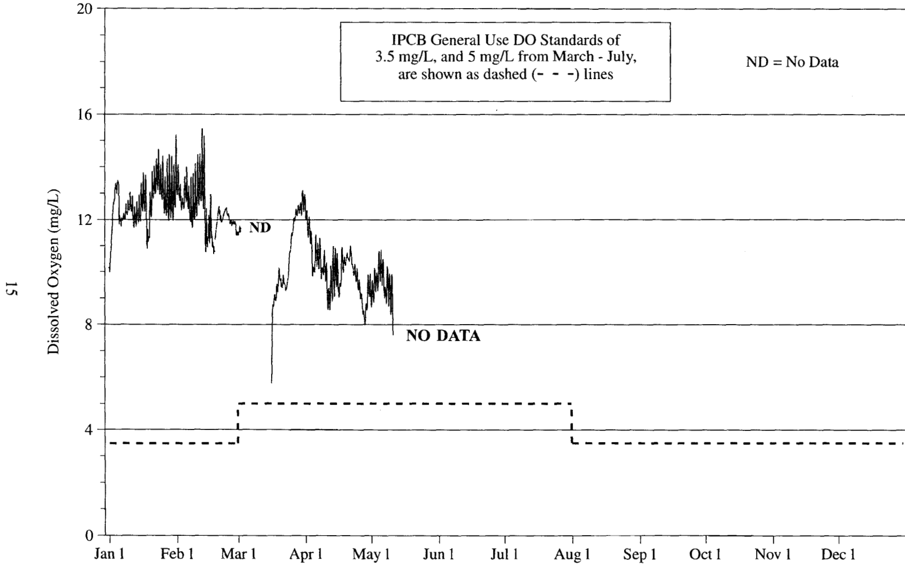
FIGURE 4: DISSOLVED OXYGEN CONCENTRATION MEASURED HOURLY AT IRVING PARK ROAD ON THE DES PLAINES RIVER FROM JANUARY 1, 2011, THROUGH DECEMBER 31, 2011
