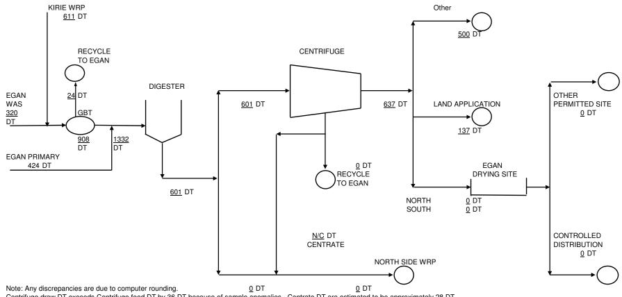
Centrifuge draw DT exceeds Centrifuge feed DT by 36 DT because of sample anomalies. Centrate DT are estimated to be approximately 28 DT.
