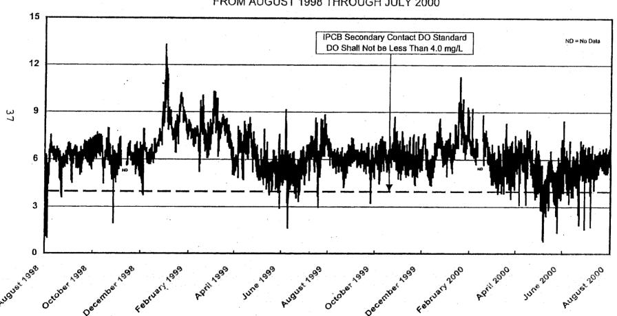
During the two-year monitoring period, DO measurements below the 4.0 mg/L standard occurred in August 1998, October and November 1998, January 1999, May and June 1999, September 1999, and April through July 2000 (Figure 13). One percent of the DO values recorded at Loomis Street were below 3.0 mg/L (Table 5).
