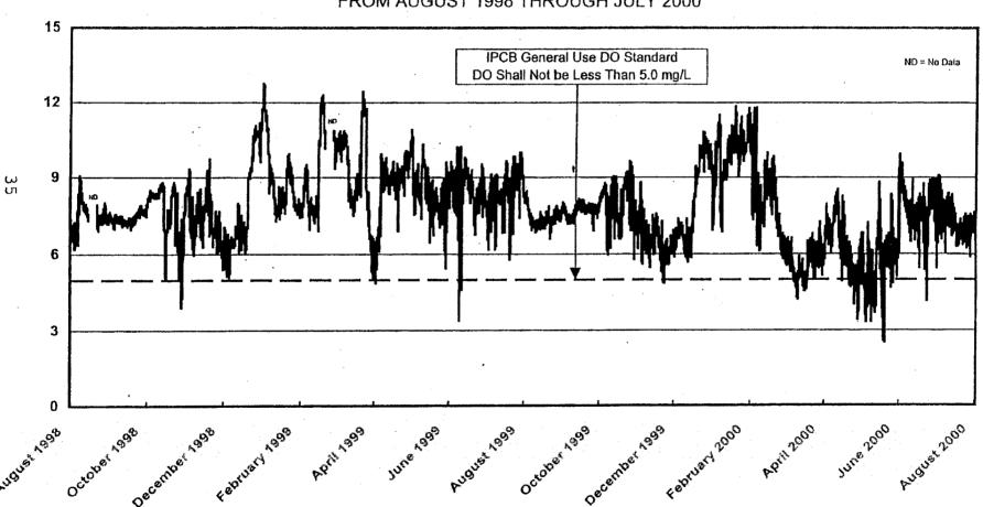
The IPCB requires that the DO concentration in the South Branch of the Chicago River shall not be less than 4.0 mg/L at any time. From August 1998 through July 2000, 16,690 of 17,061 DO values at Jackson Boulevard (98 percent) were above the IPCB Secondary Contact DO standard.
