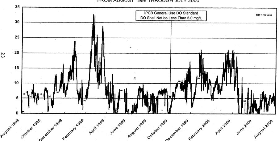
During the two-year monitoring period, DO measurements below the 4.0 mg/L standard occurred in January 1999, June 1999, November 1999, January 2000, June 2000, and July 2000 (Figure 5). Less than one percent of the DO values recorded at Devon Avenue were below 3.0 mg/L (Table 5).
