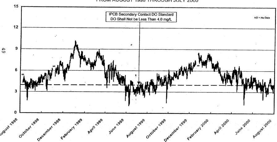
Sanitary and Ship Canal from August 1998 through July 2000 was 10.0 mg/L. The minimum DO value was 1.2 mg/L. During the twenty-four month period, the mean DO concentration was 5.2 mg/L at Lockport.
