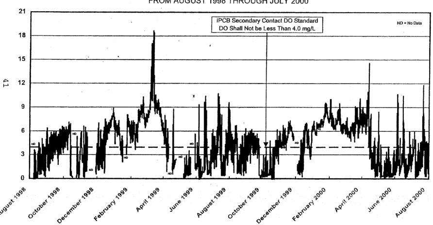
DISSOLVED OXYGEN CONCENTRATION MEASURED HOURLY AT CICERO AVENUE ON THE CHICAGO SANITARY & SHIP CANAL FROM AUGUST 1998 THROUGH JULY 2000
