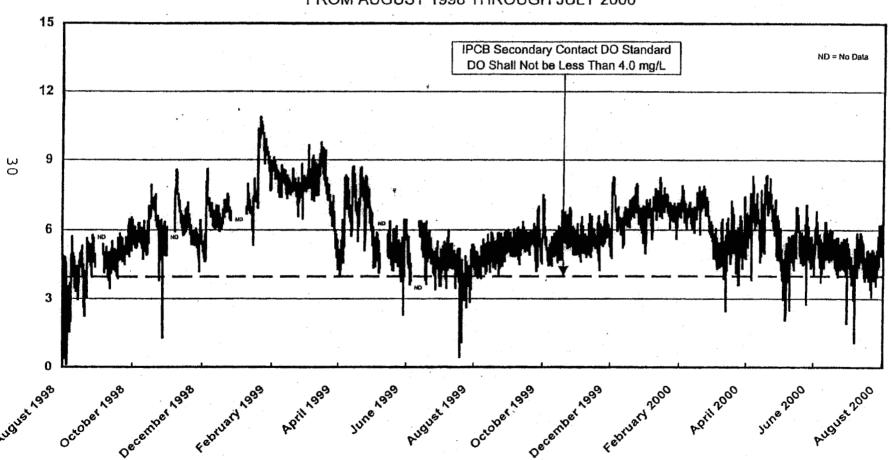
DO measurements below the 4.0~mg/L standard occurred in August through October 1998, May through August 1999, and April through July 2000 (Figure 9). One percent of the DO values recorded at Division Street were below 3.0~mg/L (Table 5).
