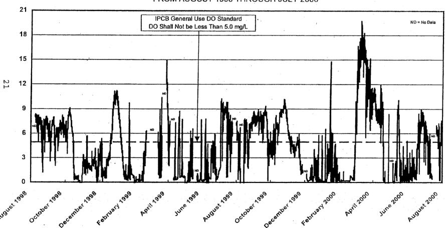
The IPCB requires that the DO concentration in those portions of the North Shore Channel classified as General Use Waters shall not be less than 5.0 mg/L at any time. From August 1998 through July 2000, 9,672 of 14,020 DO values at Main Street (69 percent) were above the IPCB General Use DO standard.
