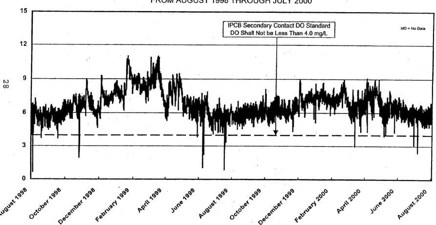
The IPCB requires that the DO concentration in those portions of the North Branch of the Chicago River classified as Secondary Contact Waters shall not be less than 4.0 mg/L at any time. From August 1998 through July 2000, 15,766 of 16,431 DO values at Fullerton Avenue (96 percent) were above the IPCB Secondary Contact DO standard.
