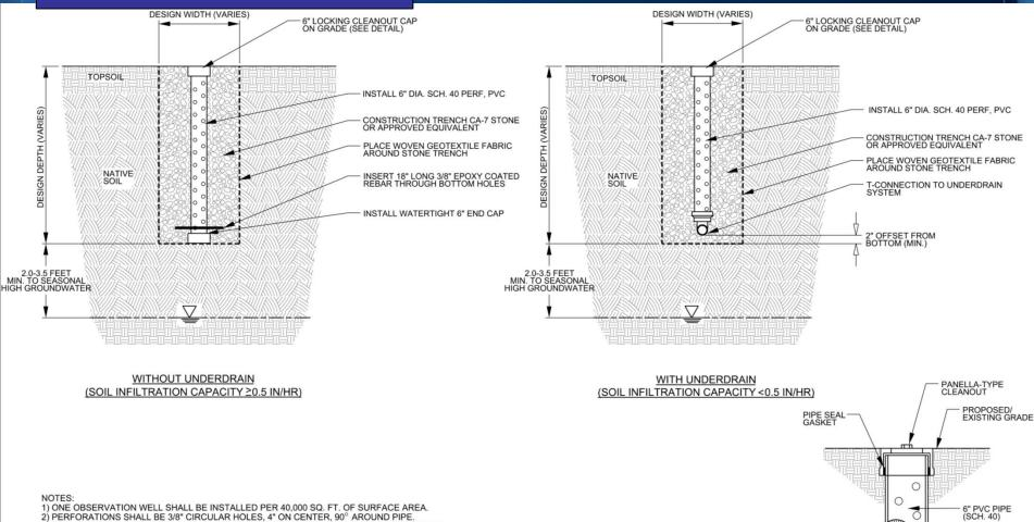
OBSERVATION WELL FOR BIORETENTION FACILITIES SHALL EXTEND 6"-12" ABOVE GRADE AND CONTAIN AN OVERFLOW GRATE INSTEAD OF LOCKING CAP.
