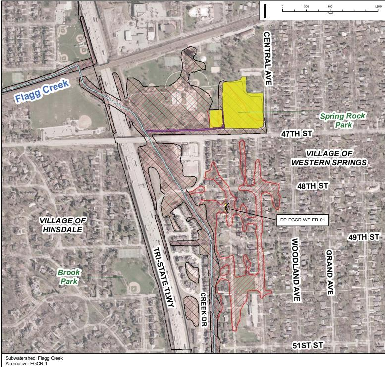
Alternatives Description: - Add and optimize storage in Spring Rock Park by lowering soccer fields appx. 8 ft. to 633 - Lower high spots to 641 in area to west of soccer fields to allow water to flow freely - Add gravity outlet with flap gate
