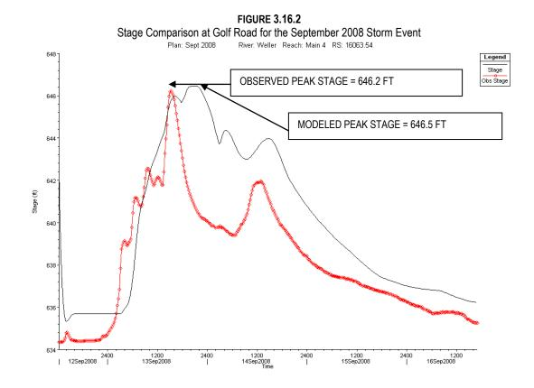
Figure 3.16.2 shows the modeled peak water surface elevation at HEC-RAS cross-section 16063.54 (Golf Road) is within 0.4 feet of the observed peak stage elevation.
