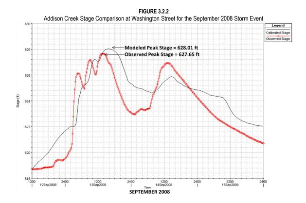
The peak flowrate of the unsteady HEC-RAS model is within 15% of the peak gaged flowrate as shown in Figure 3.2.3. The volume of the calibrated runoff hydrograph at the gage is within approximately 10% of the volume of the observed hydrograph for the September 13-14, 2008 storm event.
