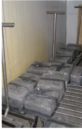
Figure 23. Slabs covered in plastic during curing.
