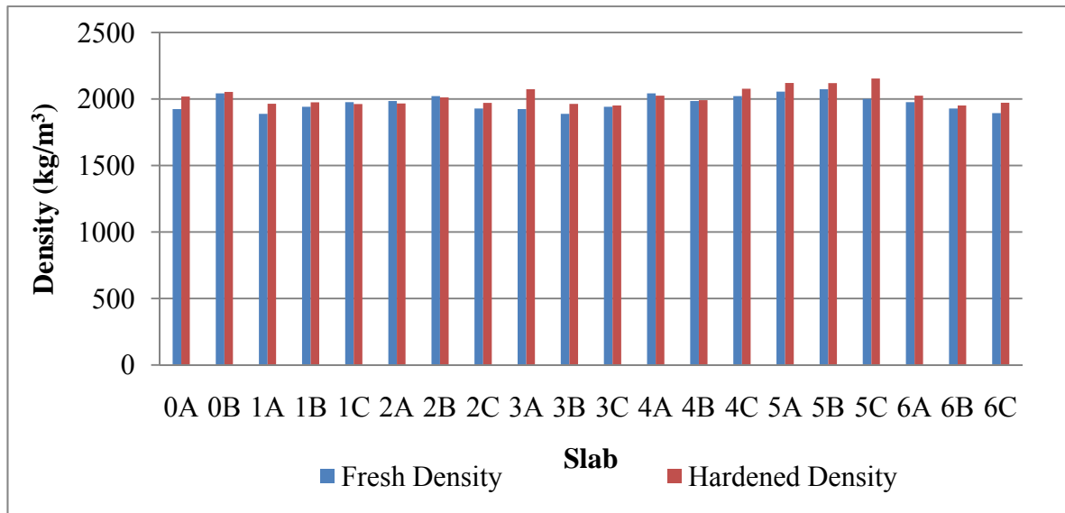
Figure 26. Density of the pervious concrete batches.
