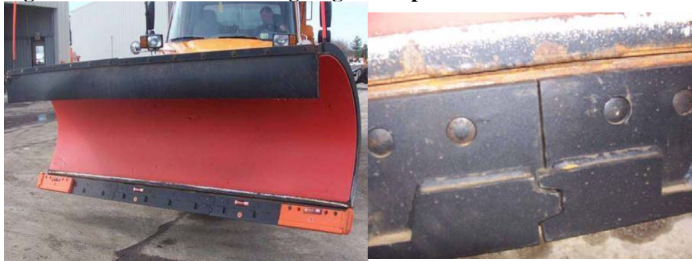
Figure 13. Razor Blade Cutting Edge Set-Up
