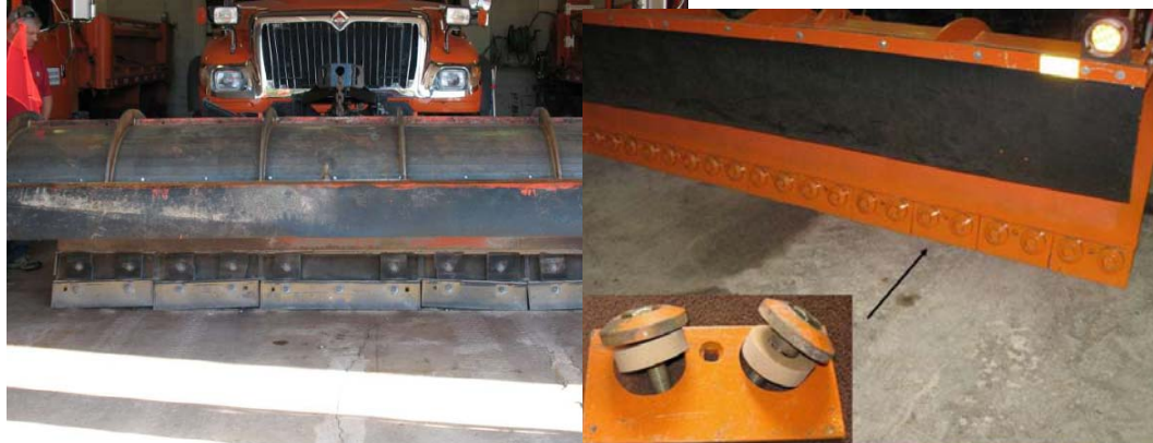
Figure 12. Flexible Edge / Segmented Blade
