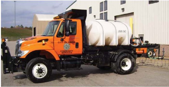
Figure 22. Liquid Anti-icing truck with spray bar
