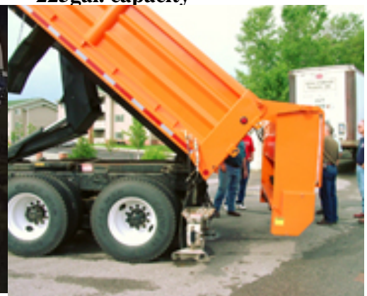
Figure 21. Integrated tailgate 225gal. capacity
