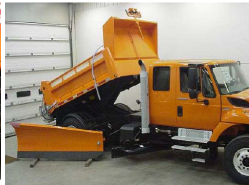
Figure 11. Dual Mid-mount wings mount wings single axle
