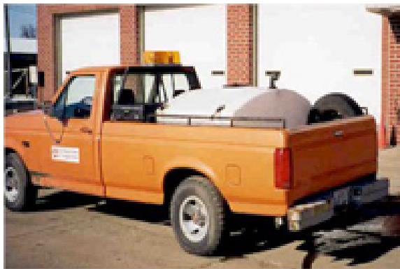
Figure 24: Slip-In Anti-Icing Brine Unit (250 gallon capacity)
