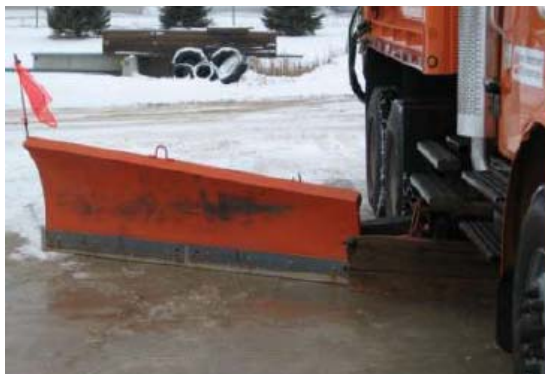
Figure 10. Underbody Plow with Mid Mount Wing Tandem-Axle
