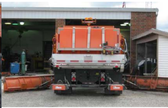
Figure 11. Dual Mid-mount wings mount wings single axle
