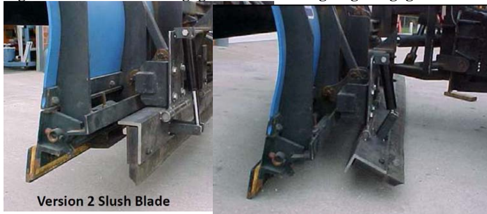
Figure 15. Slush Blade Engaged versus Cutting Edge Engaged
