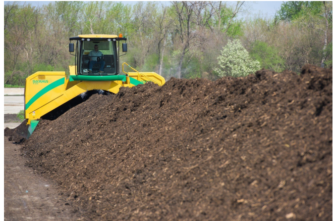
A heated windrow turns the biosolids and wood chip mixture while raising the temperature to destroy pathogens resulting in the compost product.
