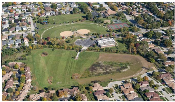
An example of the MWRD's Phase II Stormwater Management Program, the Mayfair Reservoir expansion project provides flood reduction benefits to an estimated 60 residential structures and reduces storm-related impacts for approximately 120 homeowners in Westchester. The MWRD has announced a new round of Phase II projects.
