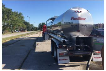
Trucks travelling significant distances across the Midwest to unload liquid waste from breweries and sugary and starch producers can now deposit that material at the MWRD's Calumet Water Reclamation Plant and improve water downstream by helping increase the recovery of phosphorus from the water stream.
