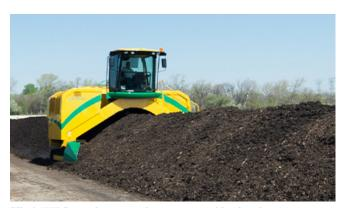
The MWRD employs a windrow turner to blend and mix its compost product that is comprised of woodchips and biosolids from the water treatment process. The blend is in strong demand during growing season and presents a victory for the environment. The MWRD has a consistent amount of this quality product now available at two convenient locations.
