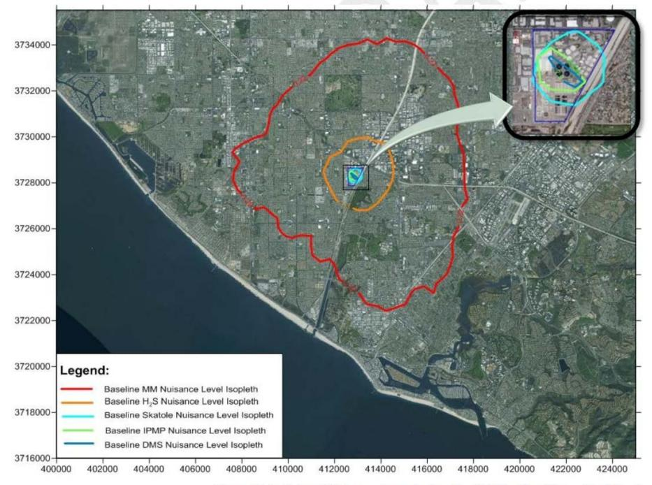
Figure ES-1. Odorant Nuisance Impacts, Baseline Existing Condition - Plant No. 1
