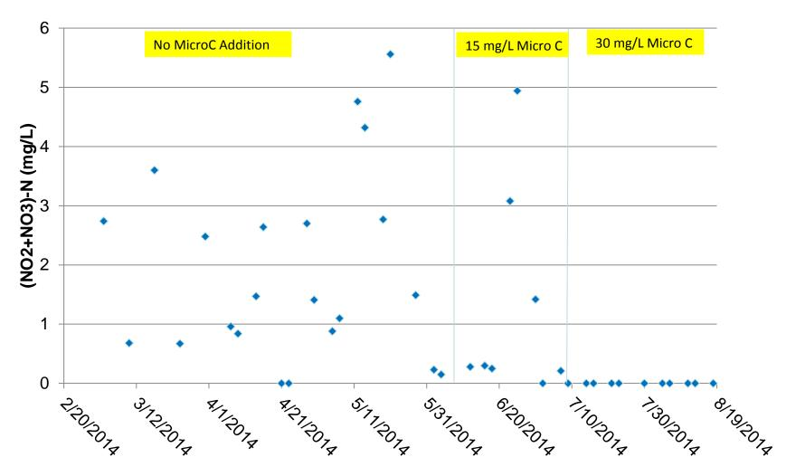
Nitrate was eliminated before the beginning of anaerobic zone-true anaerobic zone
