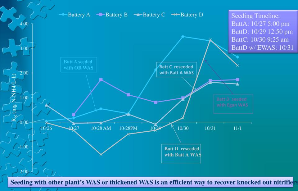
**Lessons Learned** •Plant Specific Emergency Reseeding •Real Time Monitoring of NH<sub>3</sub> Interceptor Discrete Sampling Change Early Warning Probe to End of 1<sup>st</sup> Pass
