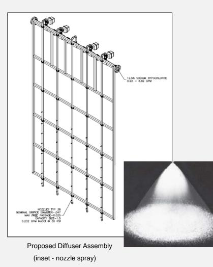
Proposed chemical diffuser system similar to systems used in the past, however, design improvements include:
