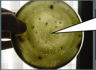
Sludge Sample Prior to WASSTRIP Implementation shows significant struvite crystals
