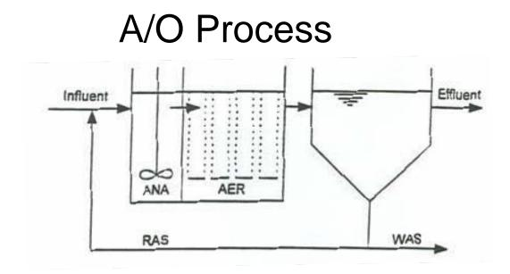
ANA = AnaerobicAER = Aerobic
