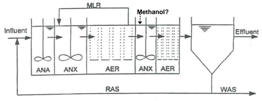
ANA - Anaerobic AER - Aerobic ANX - Anoxic MLR - Mixed Liquor Recirculation
