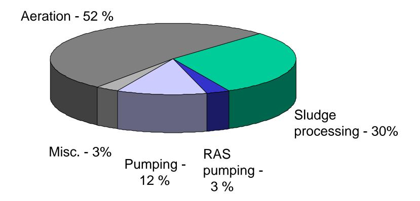
Figures shown are typical for activated sludge plants, which use approximately 1200 kWh/MG treated.
