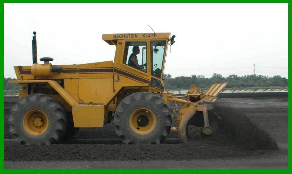
Biosolids Mechanically Agitated (Auger) During Air-Drying On Paved Drying Cells
