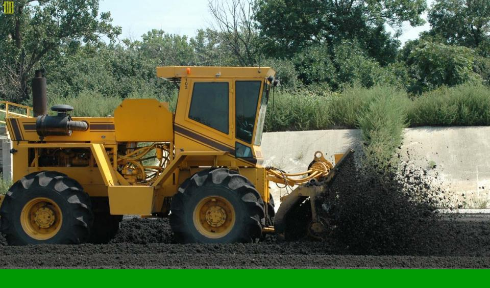
Biosolids Mechanically Agitated (Paddle Aerator) During Air-Drying On Paved Drying Cells
