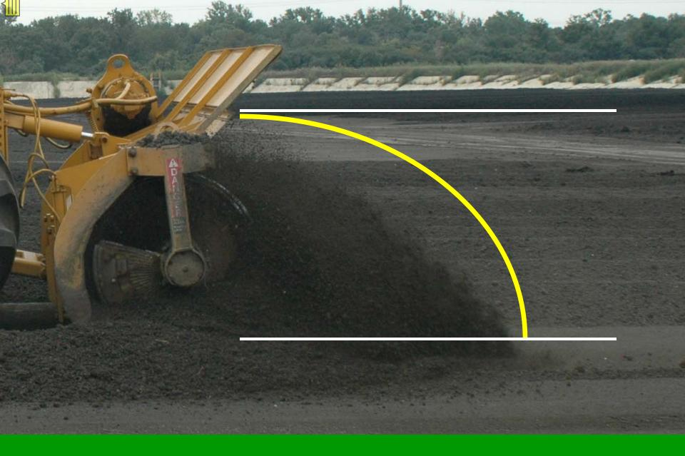
(Auger) During Air-Drying On Paved Drying Cells
