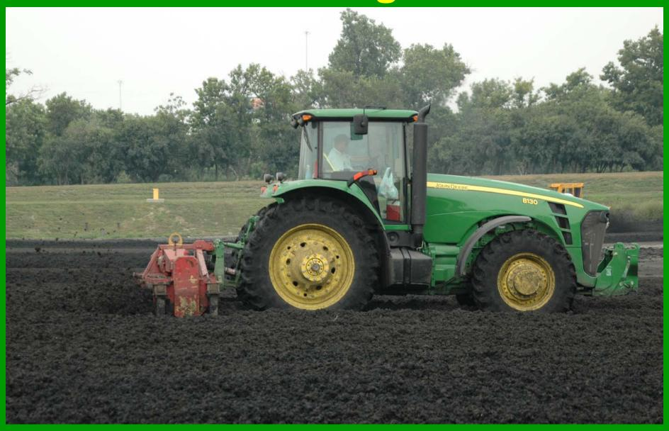
(Tractor-Tiller) on Paved Drying Cells
