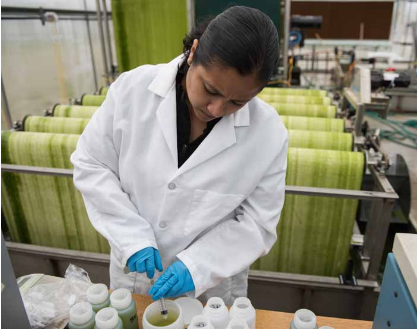
Laboratory Technician II Maricela Sabido prepares samples in the greenhouse research facility at the O'Brien WRP where the MWRD is doing research on using algae to uptake nutrients from wastewater using revolving algae biofilm reactors.
