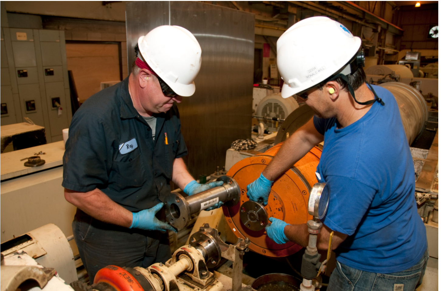
Machinists Ray Magnabosco (left) and Ron Will (right) work on a centrifuge at Stickney WRP.
