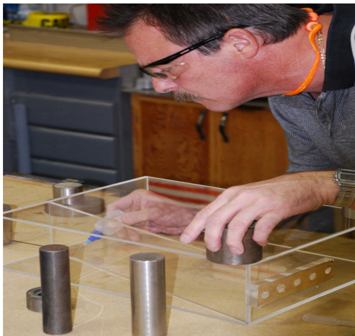
MWRD carpenter Patrick Sullivan applies an adhesive sealant while building sewer model boxes in the Stickney carpenter shop in September, 2008. The boxes replicate primary and secondary treatment processes as a part of our sewer model to be used for education and display. They will be showcased at The Field Museum Water exhibit opening in June 2009.
