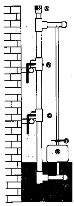
The P.V.C. Float (E) riding on the water surface will raise the indicator disk (D) to the highest water level during surcharge. The disk will remain at that level until manually reset.
