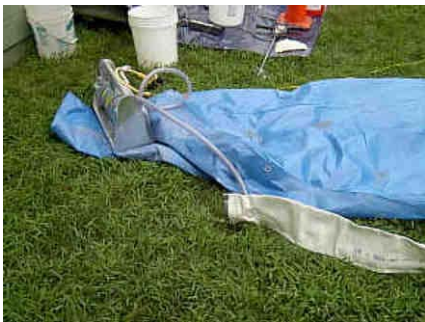
Figure A-37. Vacuum Pump Connected to the Tube.
