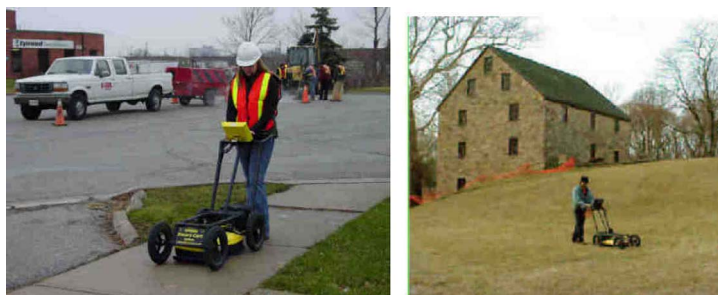
Figure 3-10. Lightweight and Compact GPR Unit (Sensors & Software Inc.).
