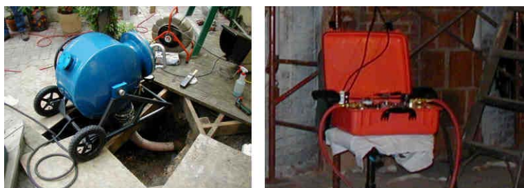
Figure C-10. Left: Inversion Drum. Right: Power Pack for Electric Curing.
