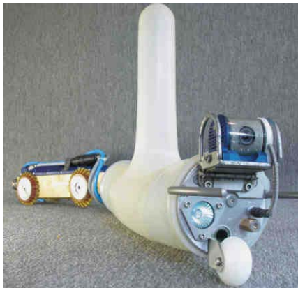
Figure A-43. Packer for Installation with Lateral Bladder Inflated.
