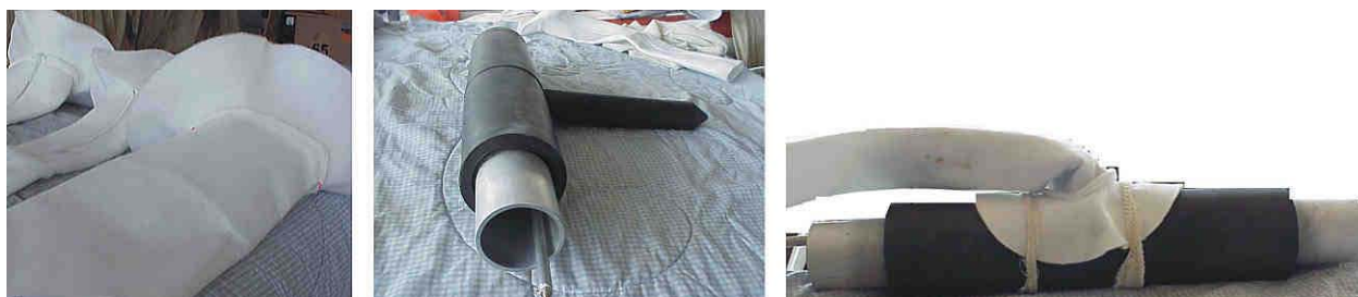
Figure C-12. Left: Material. Middle: Carrier Packer. Right: Impregnated Composite on Carrier Packer.
