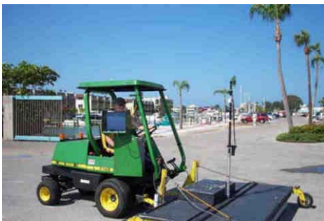
Figure 3-13. Scanning with a Mobile Array of GPR Antennae (Witten Technologies Inc).
