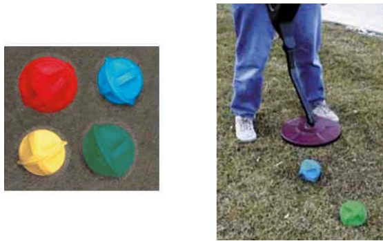
Figure 3-15. Left: Sewer Locator Balls. Right: Marker Locators for Detecting Locator Balls ( USABlueBook.com ).
