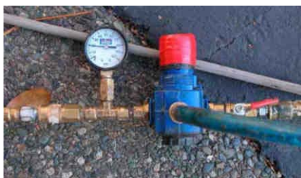
Figure A-59. The Regulator Shows the Pressure in the Bladder.
