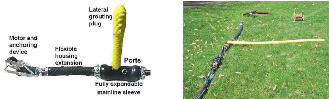
Figure 5-45. Packers Used from the Mainline. Left: Short Bladder. Right: Long Bladder—Shown Is 8' Long (American Logiball).
