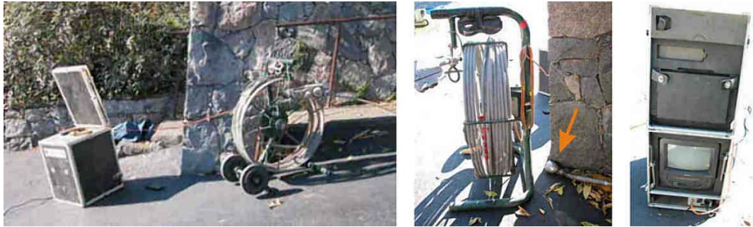
Figure A-46. Left: Portable CCTV Inspection Equipment. Middle: Orange Arrow Pointing at the Camera. Right: Portable VCR and Monitor.
