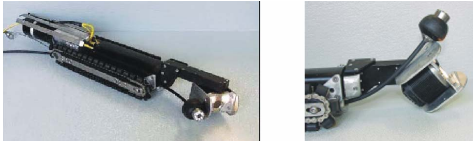
Figure B- 5. Left: RST Lateral Inspection System. Right: Close View of Lateral Camera.
