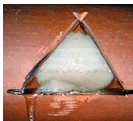
Figure 5-16. Liner Installed in Broken VCP Pipe Sample (Perma-Liner Industries, Inc.).
