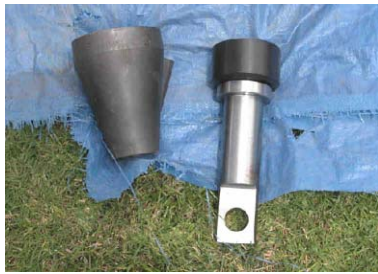
Figure 5-30. Pipe Splitting Head with Band Cutting Blade, and Clevis Head with PE End Cap (Tric Technologies Inc).
