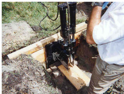
Figure A-85. Small Hydraulic Puller by Tric Tools, Inc.
