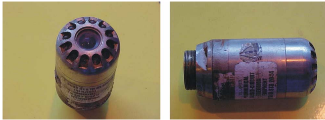
Figure 3-5. Sonde Added to a Lateral CCTV Camera (Miami-Dade County, FL).
