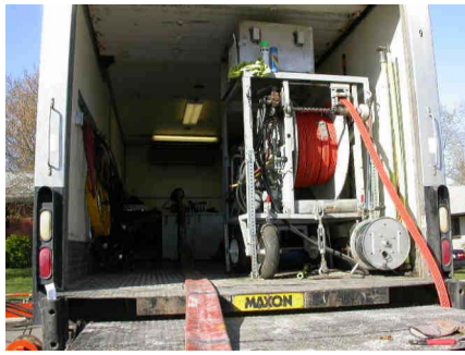
Figure A-21. Truck Used as a Mobile Wet-out Unit.
