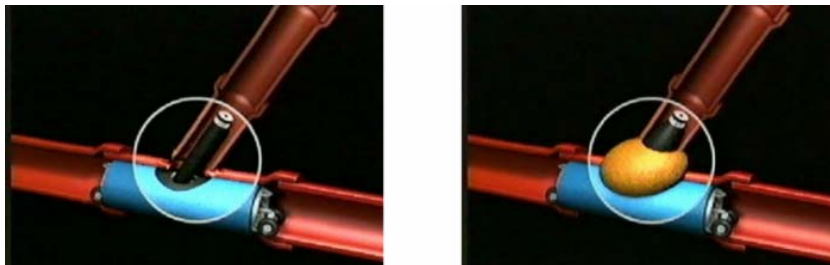
Figure 5-65. Janssen System. Left: Inflating of Bladder. Right: Resin Injection into Pipe and Surrounding Soil (The Janssen Process LLC).
