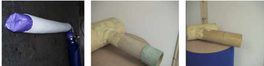
Figure C-6. Left: Liner Shown on Inverted Bladder. Middle: A 90° Junction Liner Right: A 45° Junction Liner
