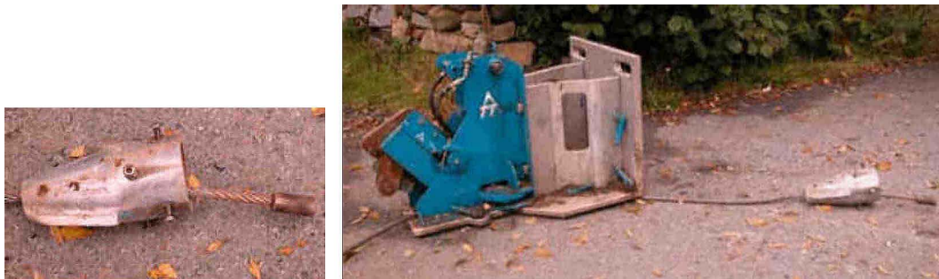
Figure A-64. Left: Nose Cone/Splitter. Right: Winch for 4" Lateral.
