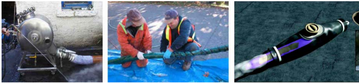
Figure 5-21. Left: Inversion Drum (Easy Liner Inc). Middle: Preparation for Insertion by Winching (Mar-Tech Underground Services Ltd). Right: Device for Inversion of Long Connection Liner (MasterLiner Inc).
