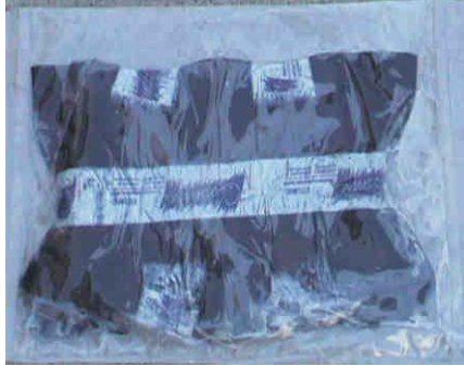
Figure A-42. Factory Impregnated TOP HAT® Delivered to Site.
