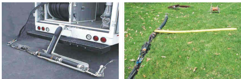
Figure C-23. Lateral Connection Packers. Left: Standard Bladder. Right: Long Bladder.
