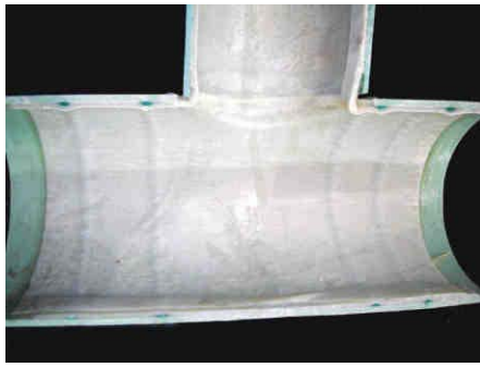
Figure 5-28. T-Liner® Installed—Cut Away Showing the 16” Mainline Seal and Hydrophilic Bands (LMK Enterprises Inc).
