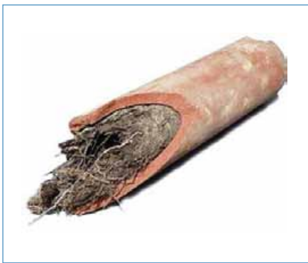
Roots intrude in the laterals, as well as sewer lines.
