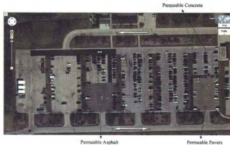
Picture 1. A picture showing relative location of permeable parking lots in an employee parking lot at the Stickney Water Reclamation Plant.
