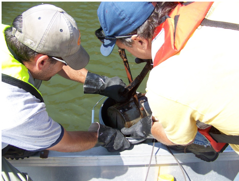
Figure 2-8: Photograph showing the Ponar dredge being retrieved from the streambed
