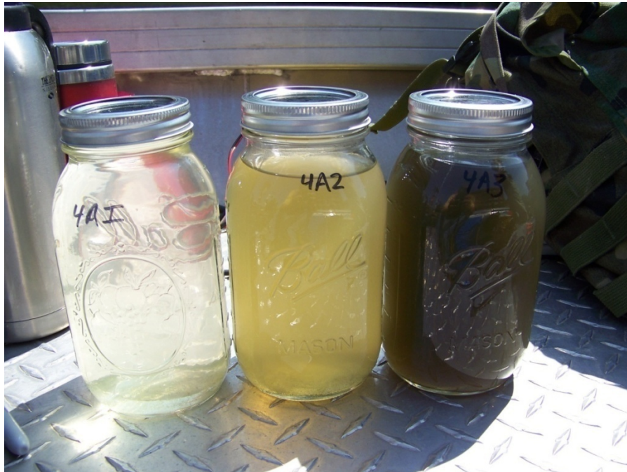
Figure 3-3: A photograph showing the different phases of resuspension observed
