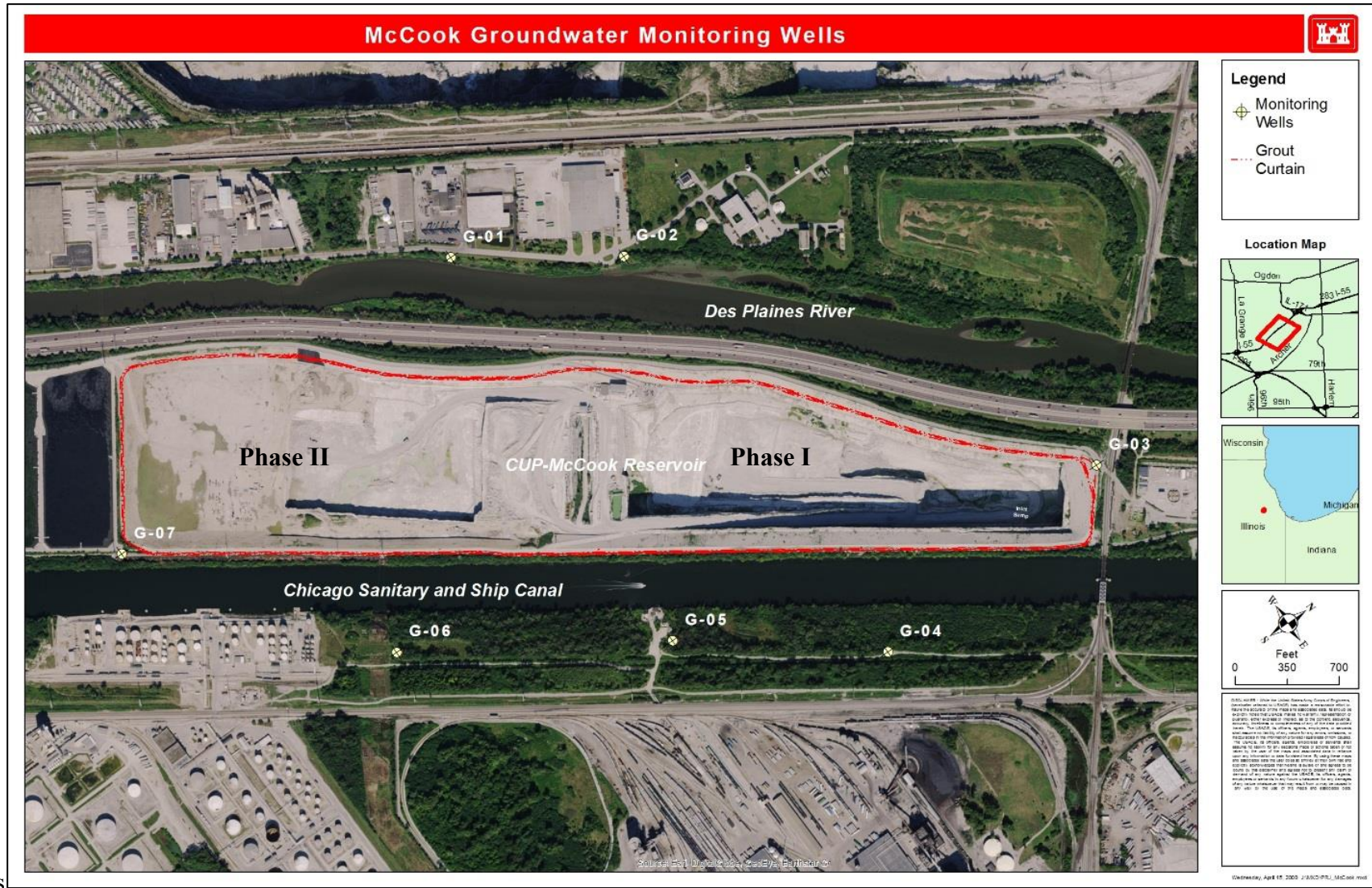
FIGURE 1: McCook Reservoir Site and Monitoring Well Locations
