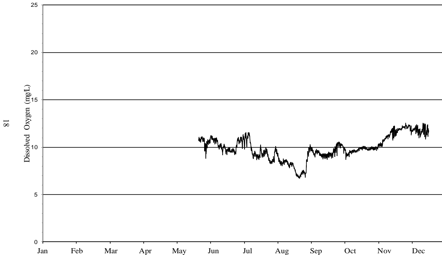
FIGURE 6: DISSOLVED OXYGEN CONCENTRATION MEASURED HOURLY AT MICHIGAN AVENUE ON THE CHICAGO RIVER FROM MAY 22, 2019, THROUGH DECEMBER 31, 2019 a
