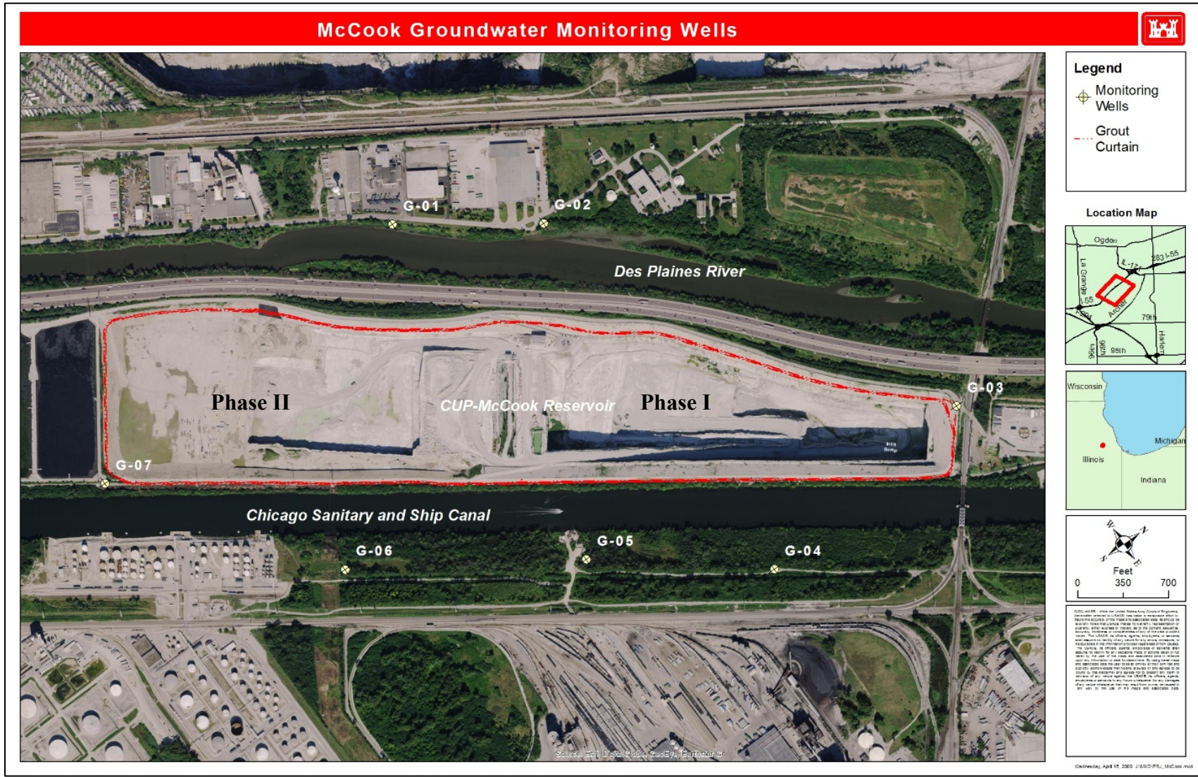
FIGURE 1: MCCOOK RESERVOIR SITE AND MONITORING WELL LOCATIONS
