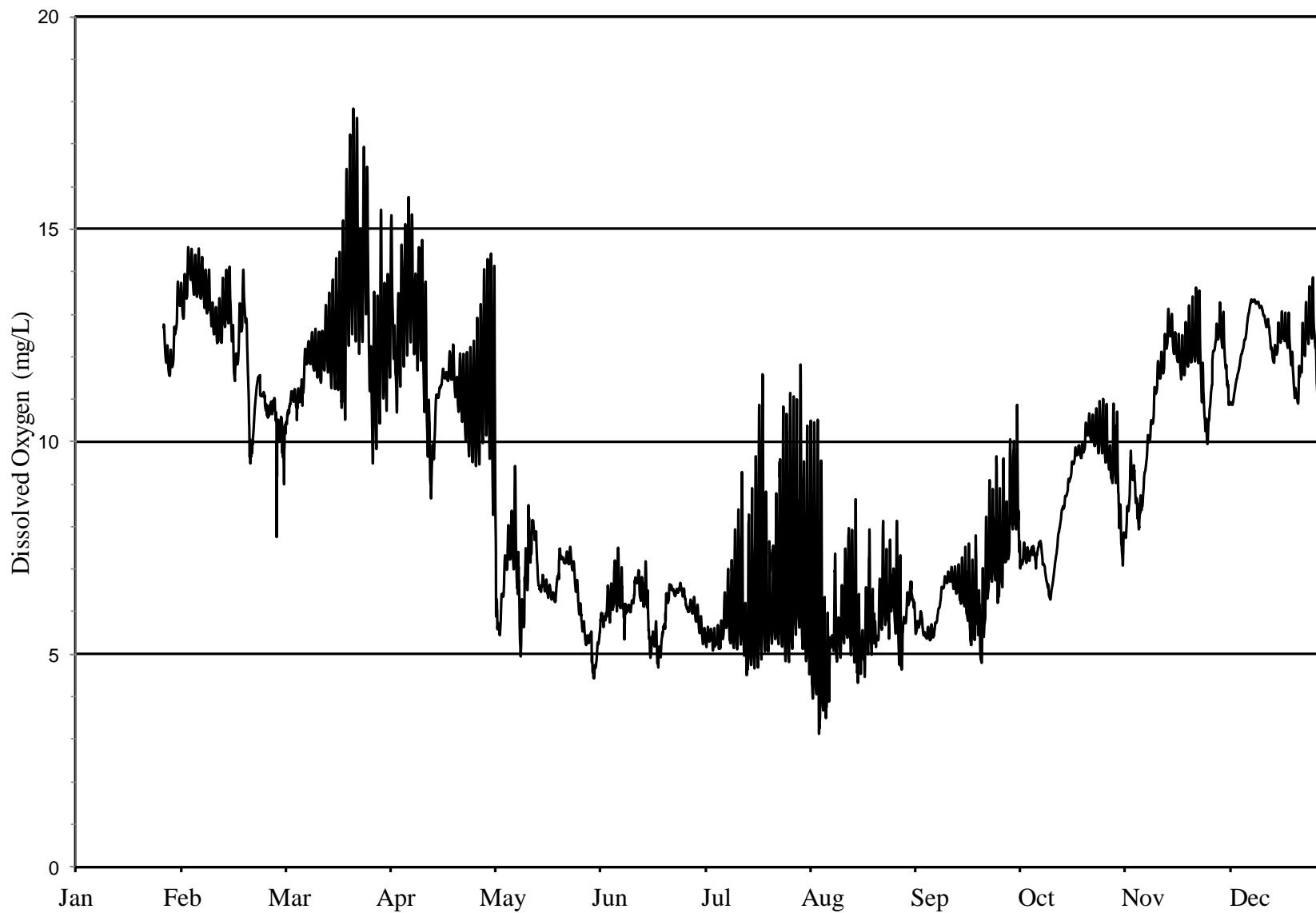
FIGURE 19: DISSOLVED OXYGEN CONCENTRATION MEASURED HOURLY AT OGDEN AVENUE ON THE DES PLAINES RIVER FROM JANUARY 1, 2018, THROUGH DECEMBER 31, 2018
