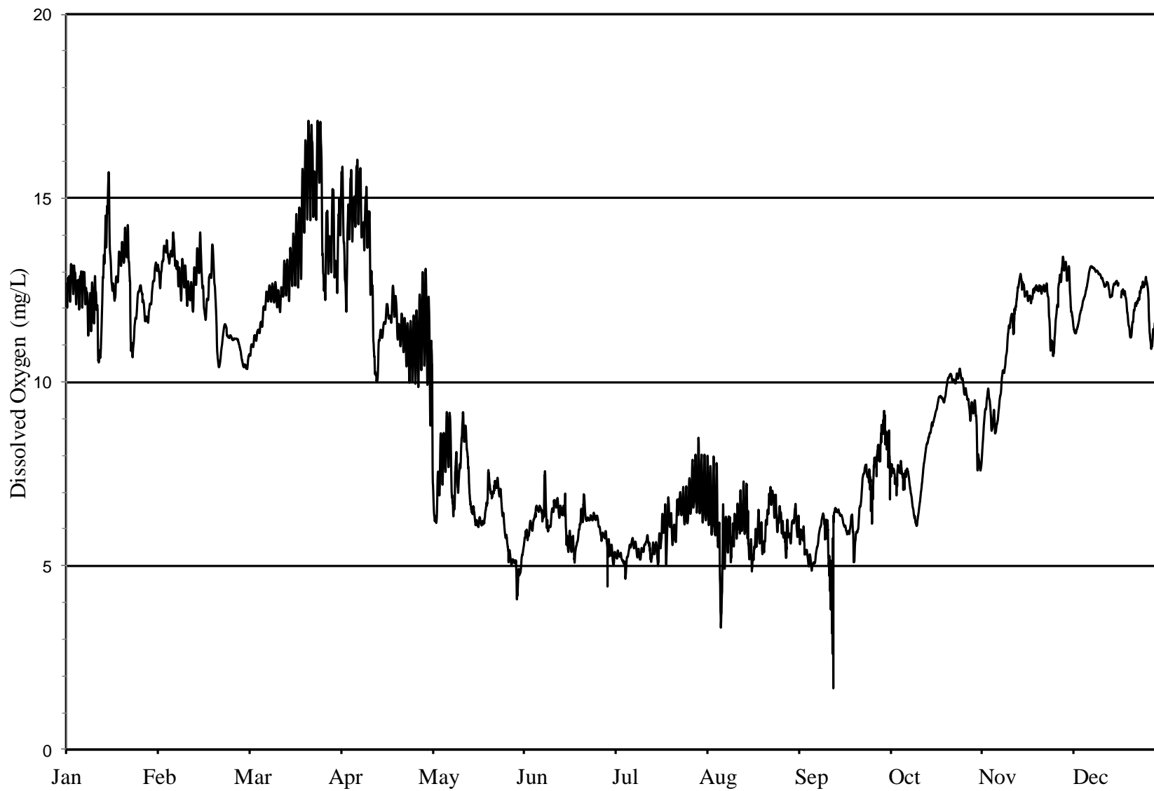
FIGURE 18: DISSOLVED OXYGEN CONCENTRATION MEASURED HOURLY AT DEVON AVENUE ON THE DES PLAINES RIVER FROM JANUARY 1, 2018, THROUGH DECEMBER 31, 2018
