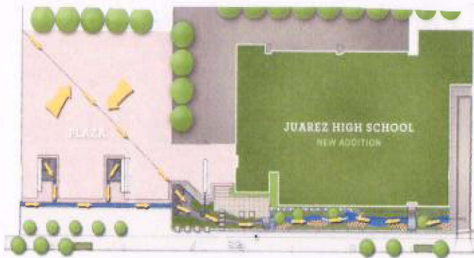
Water Feature: Arrows Indicating Overflow from Permeable Pavers in School Plaza to Bioswale
