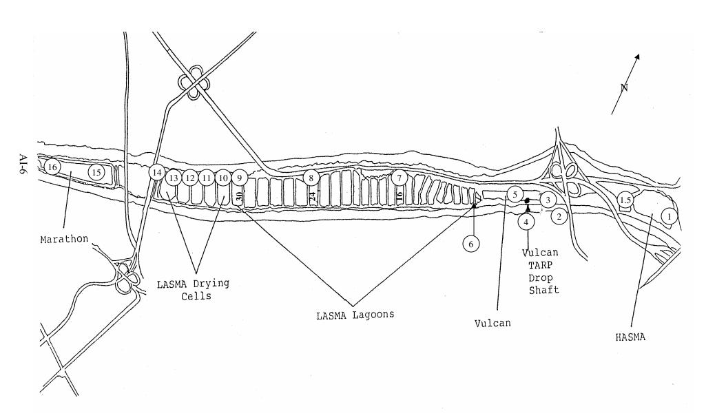
FIGURE AI-7: RIDGELAND AVENUE SOLIDS MANAGEMENT AREA SOLIDS DRYING AREA (NUMBERED CIRCLES INDICATE ODOR MONITORING STATIONS)
