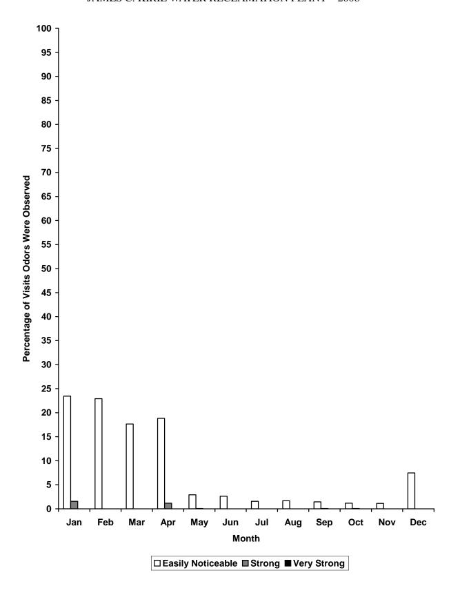
TABLE 7: HYDROGEN SULFIDE READINGS AT JAMES C. KIRIE WATER RECLAMATION PLANT—2008
