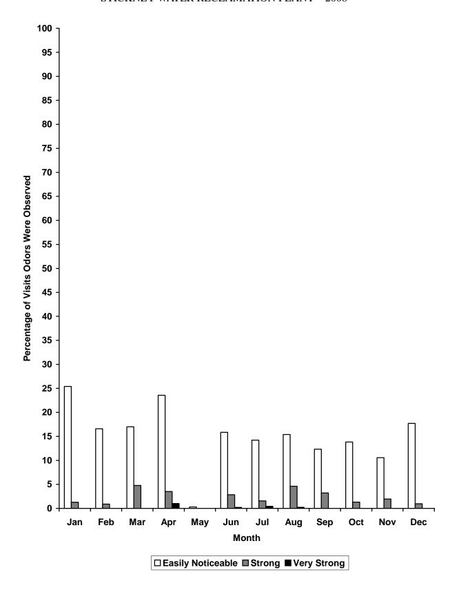
TABLE 9: HYDROGEN SULFIDE READINGS AT STICKNEY WATER RECLAMATION PLANT—2008
