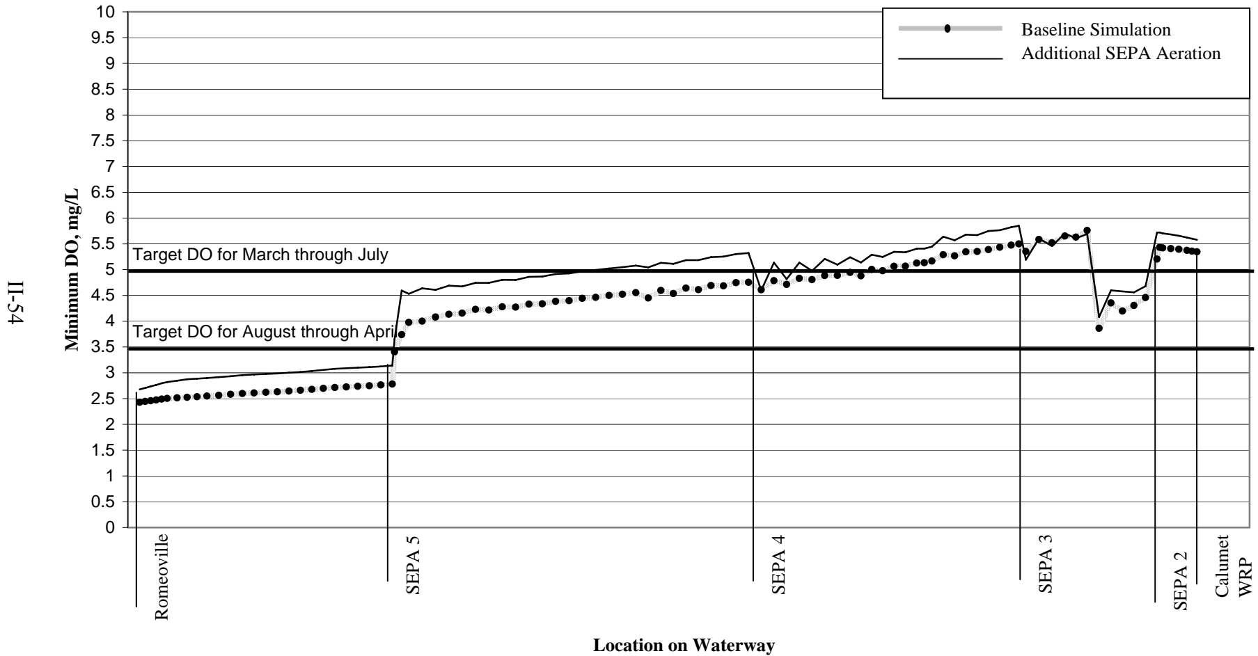
FIGURE II-5: COMPARISON OF DISSOLVED OXYGEN IN THE CHICAGO AREA WATERWAY GIVEN BASELINE AERATION VERSUS ADDITIONAL SIDESTREAM ELEVATED POOL AERATION PUMPS IN SERVICE (5/1-8/11/02)
