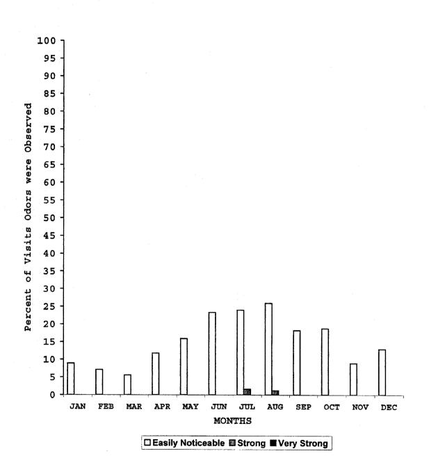
percent. The easily noticeable odors were generally in the vicinity of the waste gas burner and the primary tanks, with 22 and 30 percent of the observations, respectively, being easily noticeable. There were no strong or very strong odor observations at these locations in 2002. At the West and East Gates the odors were generally faint to no odor, 96 percent and 100 percent of the time, respectively. The easily noticeable odors were highest in the vicinity of the primary tanks.
