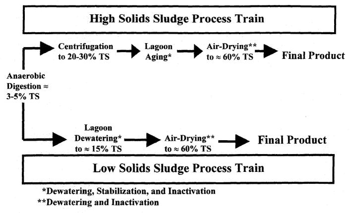
Figure 1-Sludge processing trains in the District.
