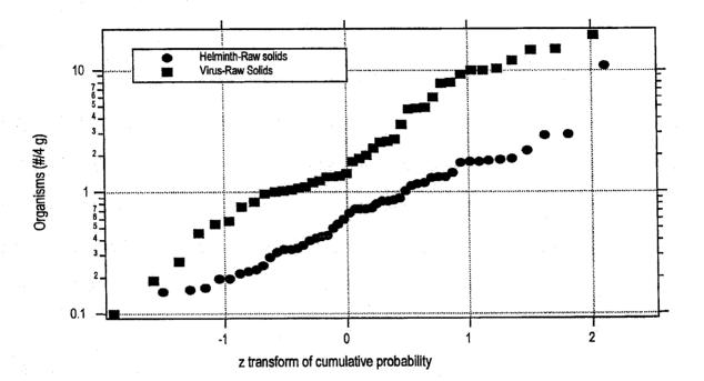
procedure was used<sup>4</sup>. The x-axis in this figure is the normal probability scale (i.e. zero corresponds to the median, and +/-1 correspond to one standard deviation away from the median value). From the figure, it is clear that the sampling period captured a two order of magnitude range in variability in influent concentrations of both helminths and viruses in the raw sludge.
