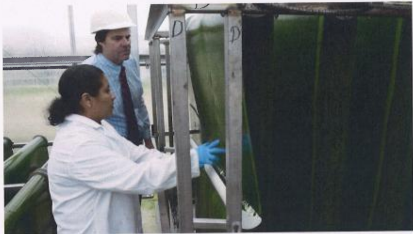
In the photo (L-R): Lab Tech I Maricela Sabido and Assistant Director of Engineering Tom Kunetz demonstrate the algae process for nutrient removal.
