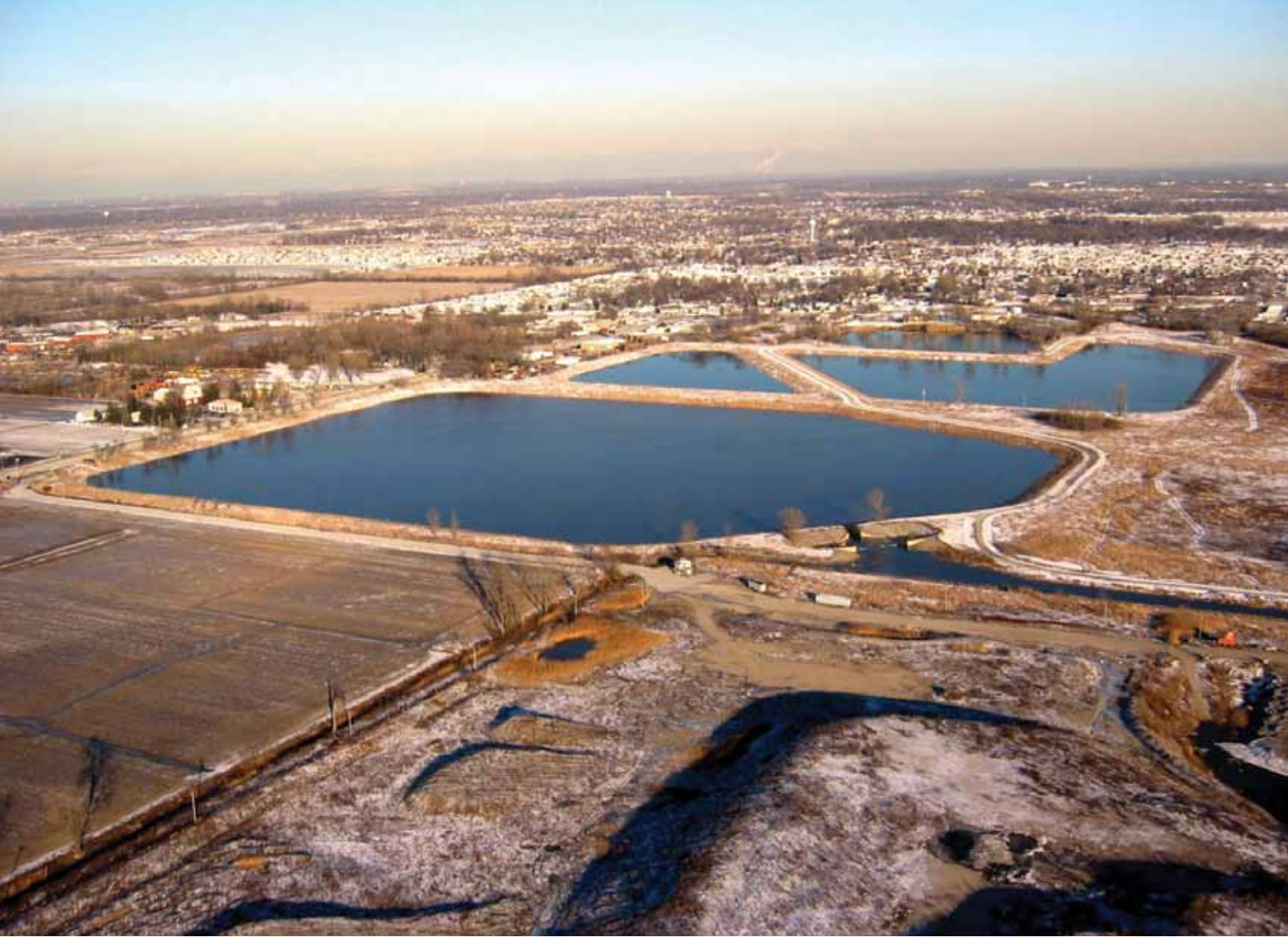
Aerial photograph of Dr. Mary Woodland Reservoir, located in Lynwood, after a storm event. This reservoir provides 351 million gallons of storage and benefits for the communities of Lynwood and Lansing.
