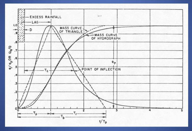
The rainfall hyetograph is used with the unit hydrograph to develop the storm hydrograph using hydrograph convolution.
