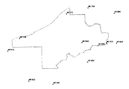
The method of surveying the Local Control Stations requires that each point be surveyed twice with different satellite configurations. If the difference in elevation between the two values is more than 10cm, the point is surveyed again until a less than 10cm difference is established between two readings. An average of the two elevations is then used as the Local Control Station Elevation.
