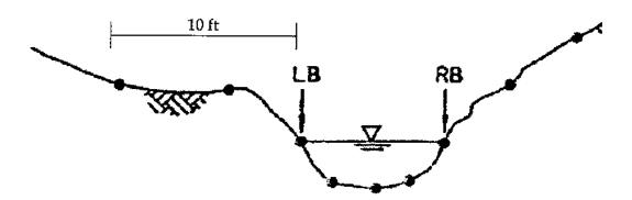
Smaller streams can use a GPS surveying method or simply submerging the surveying rod from the bank. With larger streams it is recommended the bathymetric method be used.
