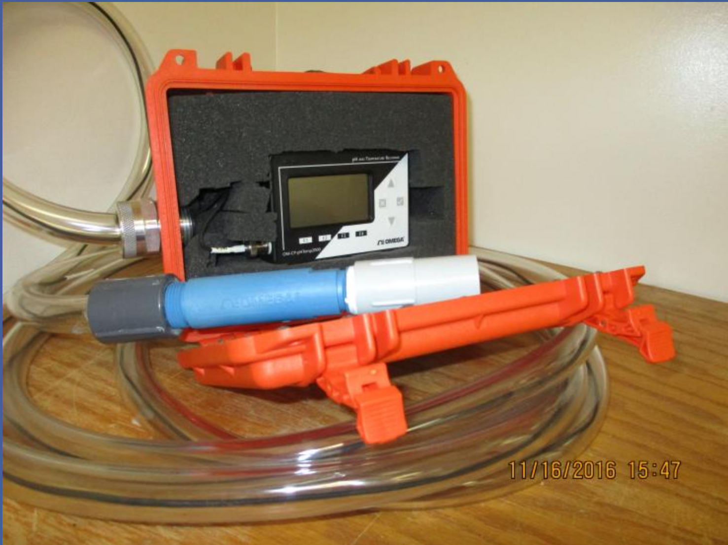
pH Loggers – Deploy in Manholes Outside Industries
