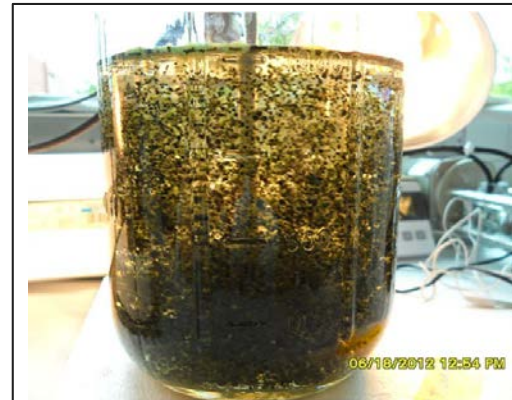
Biogranules mixing in an SBR during light reaction period.
