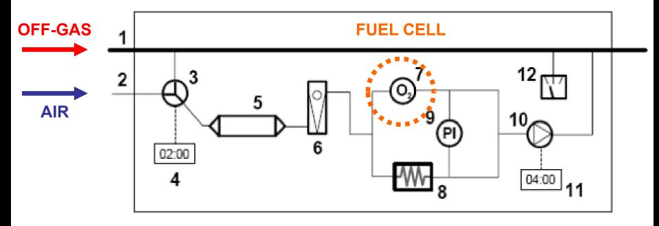
Key: 1) off-gas hose (from collection hood); 2) reference air intake; 3) three-way valve; 4) time delay relay; 5) column for CO<sub>2</sub> and H<sub>2</sub>O removal; 6) flow meter; 7) oxygen fuel cell; 8) resistance; 9) differential manometer; 10) vacuum pump; 11) time delay relay; 12) air velocity meter. Solid lines = hydraulic line, dashed lines = electrical connection
