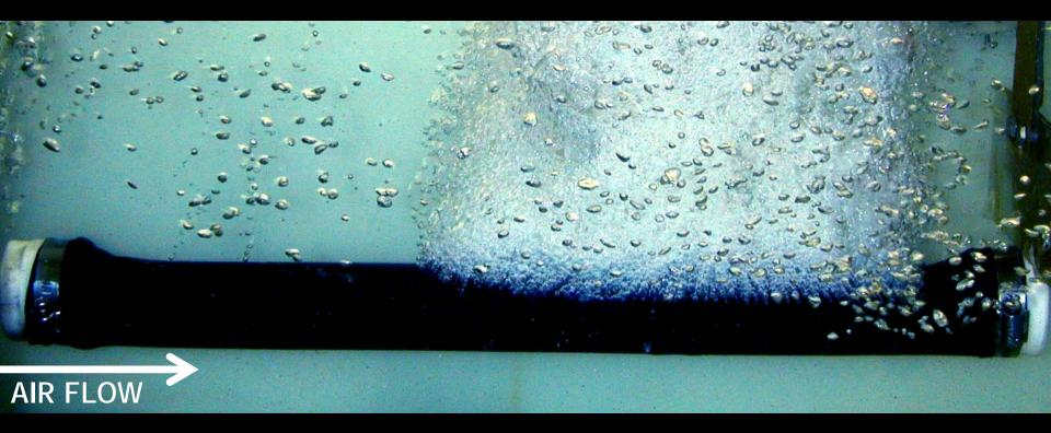
Orifice creep caused sludge to enter the diffuser and form a crust inside
