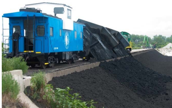
Biosolids are delivered by train from the Stickney Water Reclamation Plant to the Lawndale Avenue Solids Management Area, where they are mixed with wood chips to produce high quality compost.
