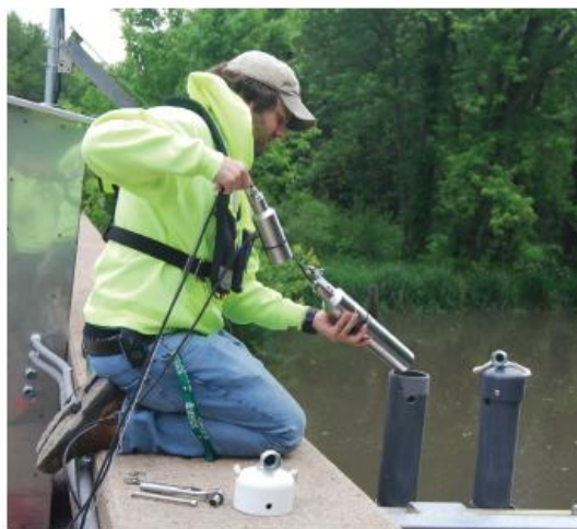
Colin Peake installs a nitrate sensor at a U.S. Geological Survey super station site. Kelly Warner, U.S. Geological Survey Illinois Water Science Center
