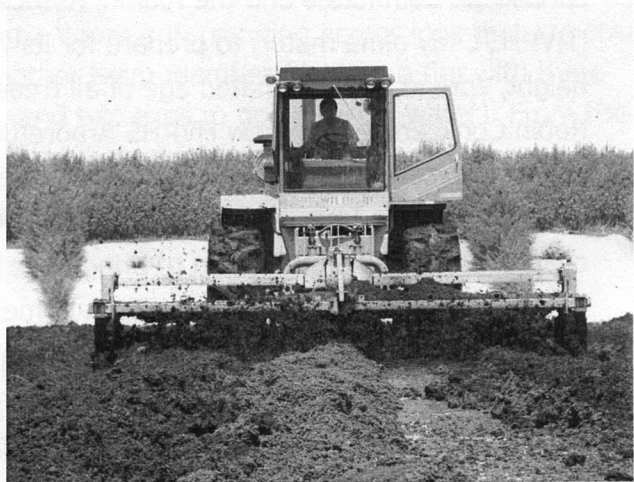
Turning windrows of mixed biosolids and waste wood
